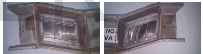
Figure (15): CFRP Separation in both shear zones without slippage for beam (04-SCLVA)
