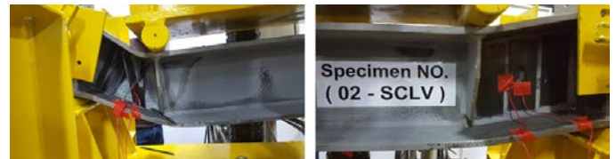
Figure (13): CFRP separation in left shear zone for beam (02-SCLV)
