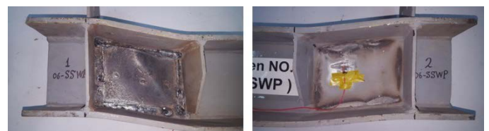
Figure (17): Shear buckling of the steel web with a failure beside the welding area in left shear zone (beam 06-SSWP)
